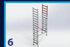
**3:** Attach the 1st horizontal brace with red trigger to the upright above the bottom rung of the top gate frame. Fit to the collars of the adjacent frame and repeat with second brace
