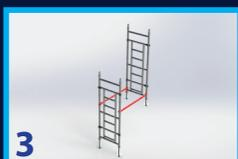
**7:** Attach a diagonal brace with blue trigger from the 9th rung of the bottom frame to the 9th rung of the top frame. Attach the platform to the 8th rung of the top frame and the 12th rung of the bottom frame. Ensure the platform is secure and level and then lock the wind clips. If using stabilisers fit at this point, if not tie or buttress to the stairwell
